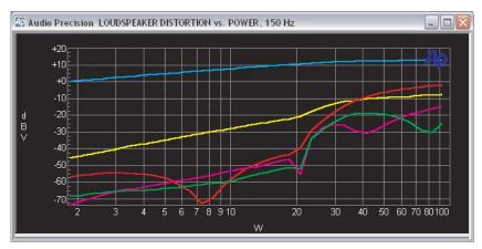
Figure 328. Fundamental (top curve), 2nd harmonic, 3rd harmonic, 4th harmonic, and 5th harmonic amplitudes of a loudspeaker as a function of power.
